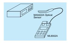
The MA9422A Optical Sensor is only 3 mm thick at the tip so it can measure power in confined places.
