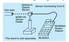
The optical sensors can be used remotely from the mainframe with the MA9006A Sensor Adaptor, MZ8013A Sensor Holder and Sensor Connecting Cord S.
